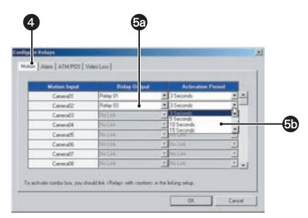
Figure 130. Linking Relays to Motion Detection
